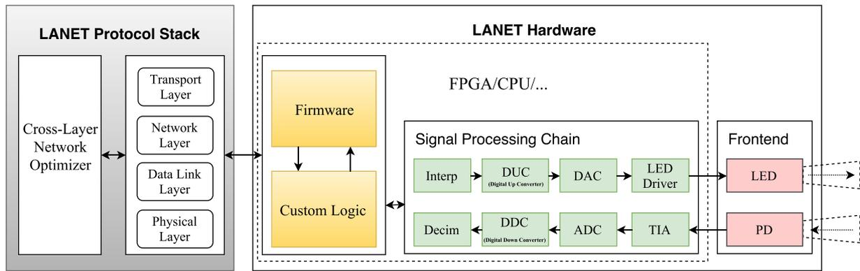
Fig. 2. Reference Architecture of LANET Node.
