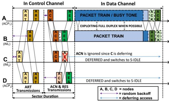
Fig. 3. Timing diagram of VL-MAC.
