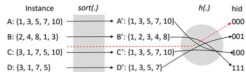
Fig. 3: Illustration of hash mapping.
