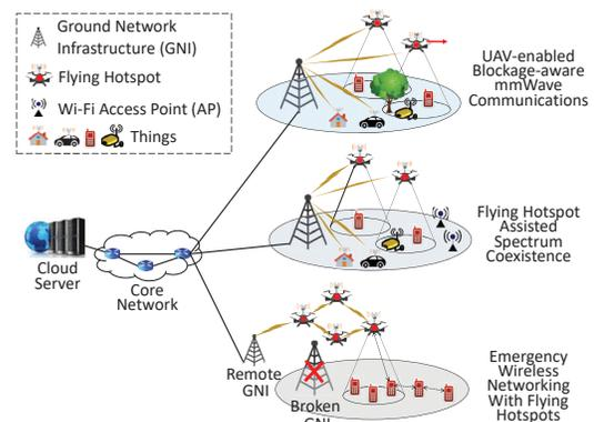
Fig. 1. Applications of UAV-assisted wireless networking.
