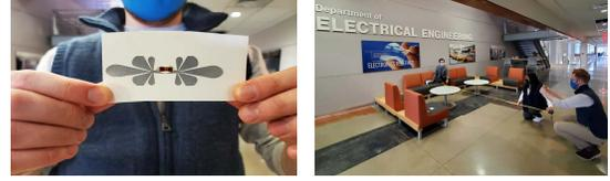
Fig. 6: Snapshot of experiments. (Left) printed antenna Ant-5-100-10; (Right) read range measurement.
